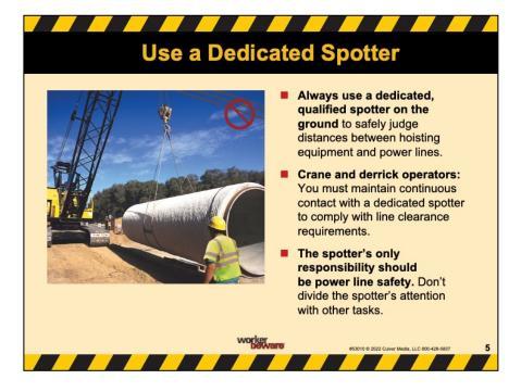
Use a dedicated spotter when working with hoisting equipment around overhead lines.
