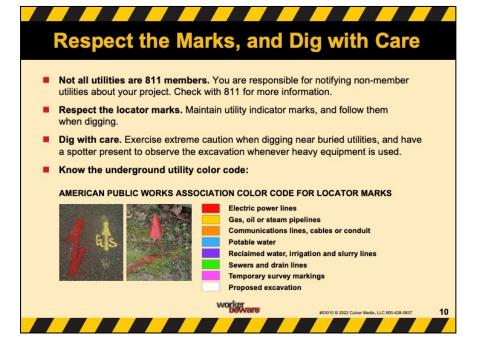
After you contact 811, the underground utility locator service will arrange for each member utility to send someone out to your dig site to mark the underground lines.
